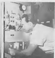
NEW MICRO vapor pressure apparatus determines v.p. of gasolines and jet fuels. Operator is Thomas Halley.
